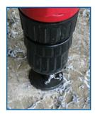
**4.** The guide will direct the cutter; the stop will touch when completed.
