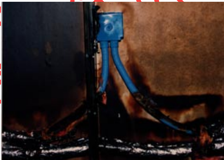
Figure 44: ASTM E-119 ENT box installation after 30 min. fire exposure
