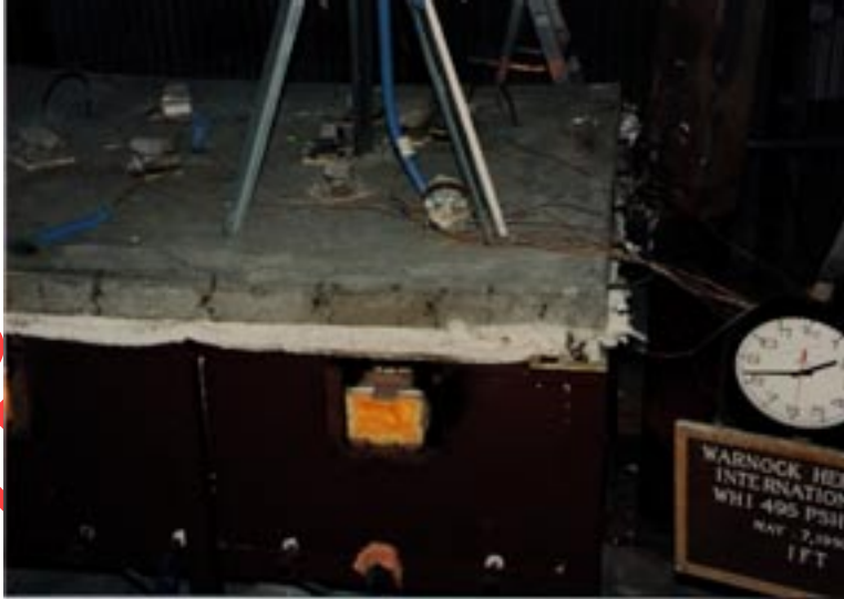
Figure 36:2-hour ASTM E-119 slab exposure
