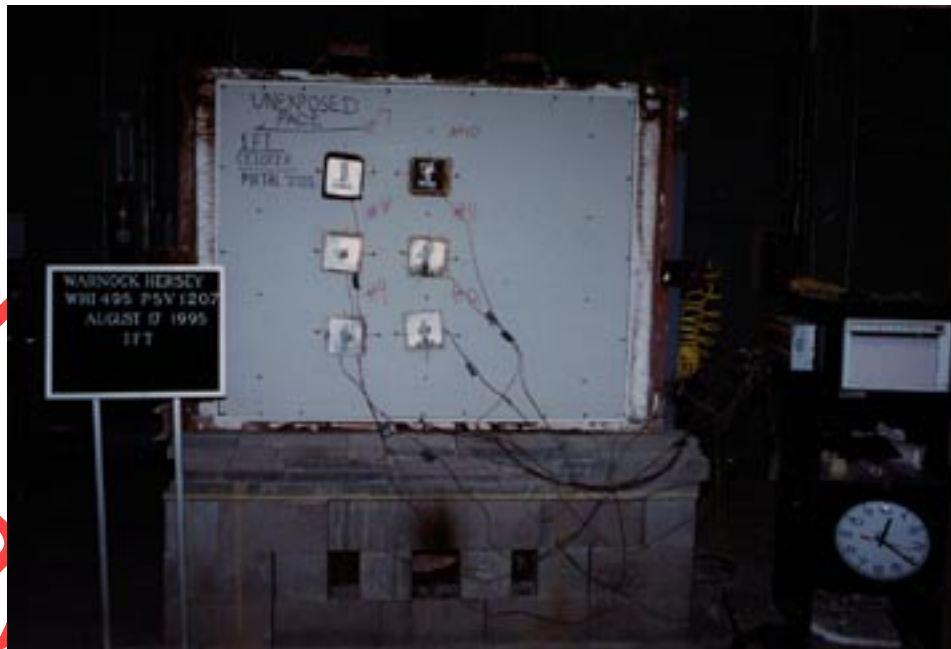
Figure 40: Per previous photo during ASTM E-119 furnace exposure
