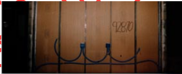
Figure 41: ASTM E-119 30 minutes hose stream specimen prior to fire exposure
